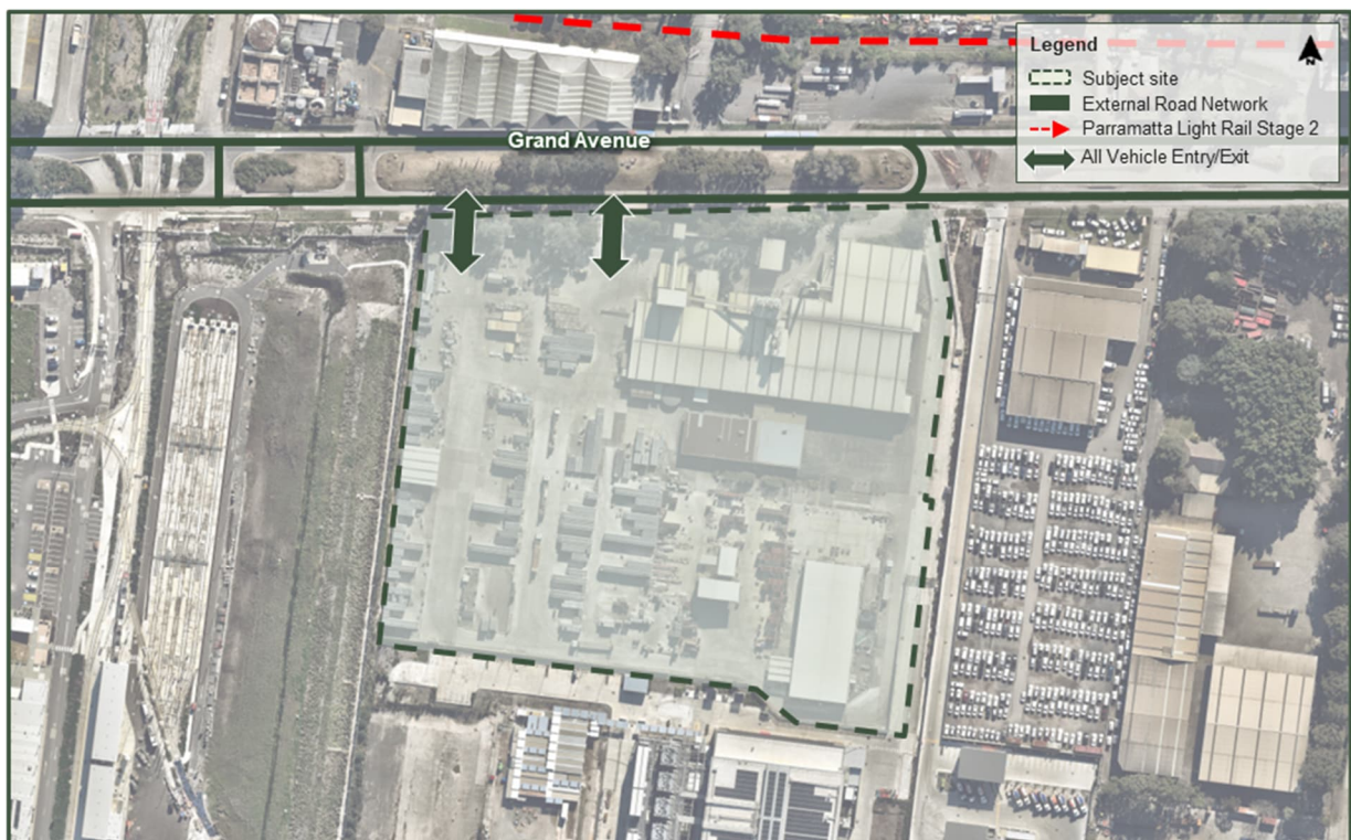
Figure 3 Construction Access Arrangements
